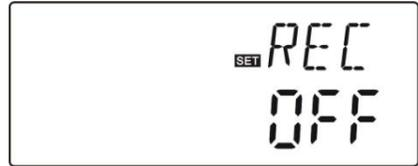
▶ Re-press "SET" button to activate or deactivate this function, after function activated; factory set is "REC ON"
