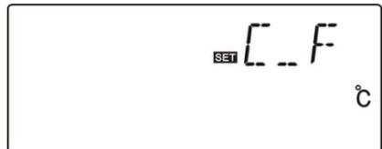
▶ Press "▲" button, to select between Celsius and Fahrenheit temperature, factory set is °C
