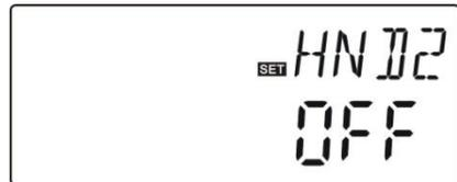
**Note:** when manual mode is
