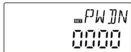
▶ Press “SET” button, “PWDG 0000” displays on the screen, ask for reentering the new password, doing like above to reenter the new password, “PWOK” displays on the screen to indicate reentering password successfully.
