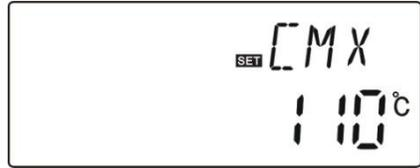
▶ Press “ESC” button to exit the menu or wait for 20 seconds to exit automatically, parameters are saved automatically.
