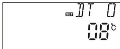
▶ Press "▲ ▼" button, to adjust the value of switch-on DT, adjustable range (OFF+2°C) ~20°C, factory setting is 8°C
