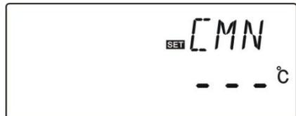
▶ Press “ESC” button to exit the menu or wait for 20 seconds to exit automatically, parameters are saved automatically.
