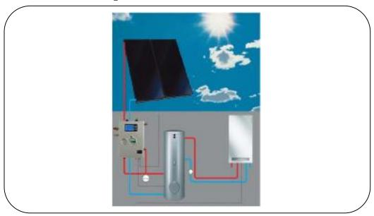
SP226 should be installed in forward flow (manometer side) and return flow (pump side) of the solar circuit, as indicated above. Please see detailed installation instruction in attached manual.
